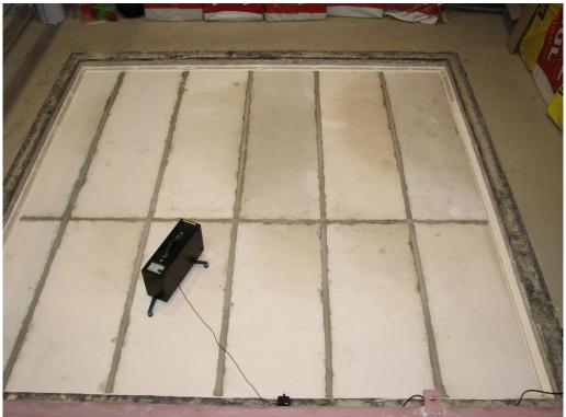
Figure 2 : Test setup of impact machine on floor panel system
