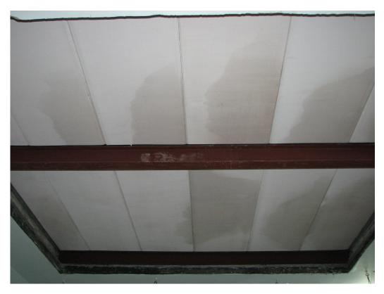
Figure 3 : Test setup of floor panel system installed on top of the reverberation room
